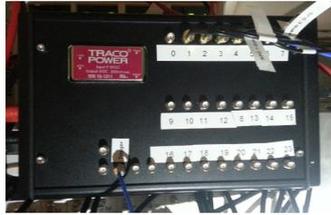
**Figure 2.23:** Photo of the Pulse Generator. This FPGA-based device can output TTL pulses with a sample rate of 1 GHz on 24 channels.
