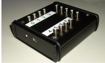
**Figure 2.25:** Photo of the Time Tagger, an FPGA-based device which allows the detection of TTL pulses with a resolution of 60 ps on 8 input channels. The detection can start with an external trigger and arrays of time-binned counts can be generated for convenient data analysis.
