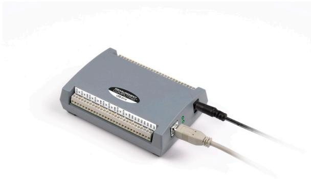
**Figure 2.27:** Photo of a 16-channel highly stable voltage source. Each channel has 16 bit resolution over  $(-10 \text{ to } 10) \text{ V}$ . It is programmed automatically according to variables specifying the voltages in the computer control user interface. Image courtesy of Measurement Computing.
